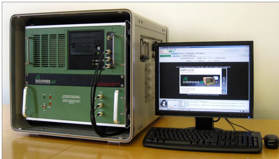
Figure 4.3 - The Digital Portable Sounder (DPS4D) with a computer system running the Digisonde software.
