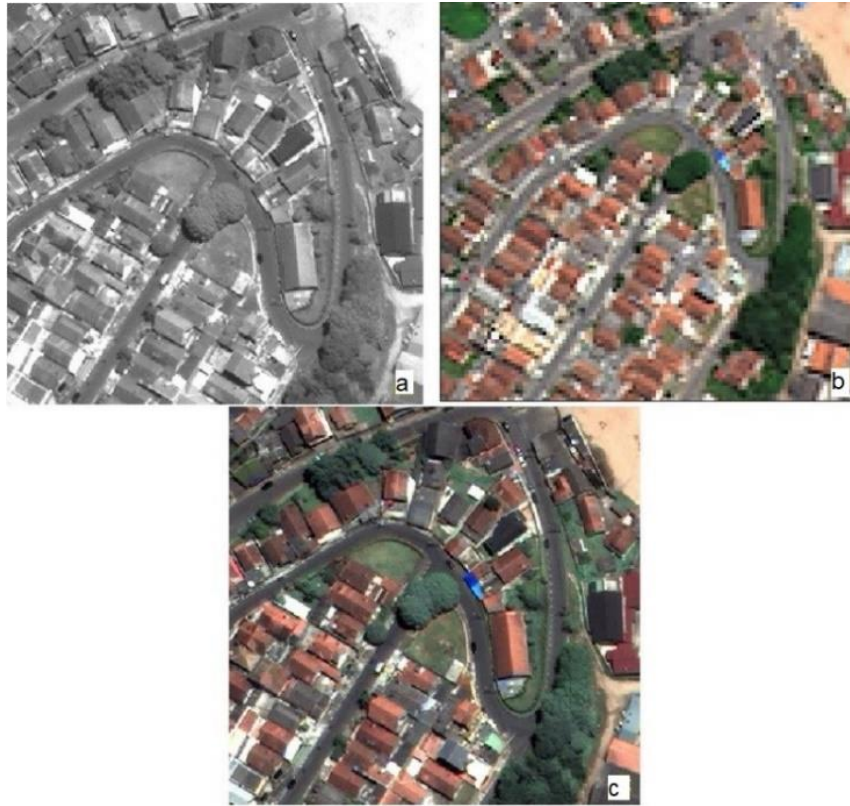
Figure 5.2. Example of pansharpening procedure using Gram-Schmidt method with IKONOS image: a) panchromatic band, b) multispectral band and c) pansharpened image.
