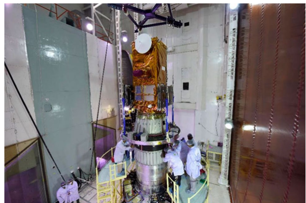
Fig. 1 Amazonia 1 satellite assembled on PSLV fourth stage (Source: INPE/ISRO)
