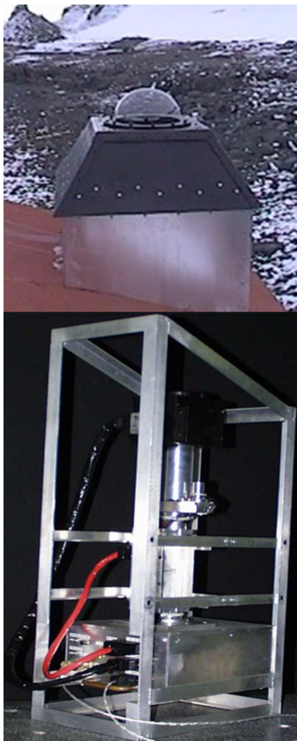
Figure 1. Glass dome at the roof of Punta Plaza shelter (top) used to house the FotAntar-1 instrument (bottom).
