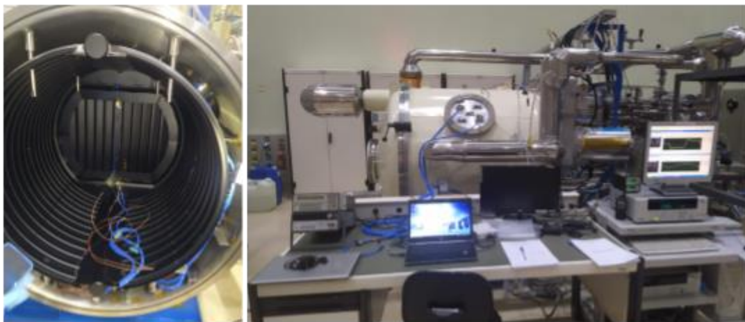
Figure 6: EDC installed inside the thermal vacuum chamber (left). On the right, functional test setup used during the thermal vacuum test.
