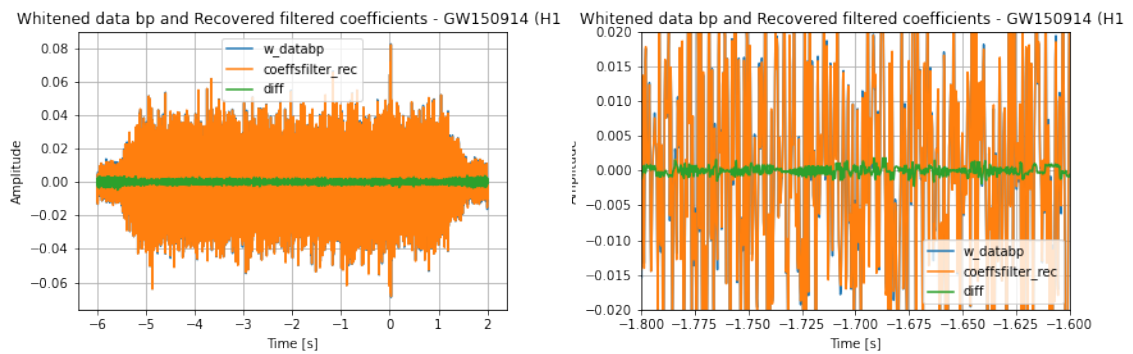
Figure 5.19 - Inverse Discrete Wavelet Transform for the GW150914 (H1) coefficients filtered with quantile and a bandpass filter ([20,1000]Hz). The difference between both original and IDWT filtered data is represented with the diff curve.
