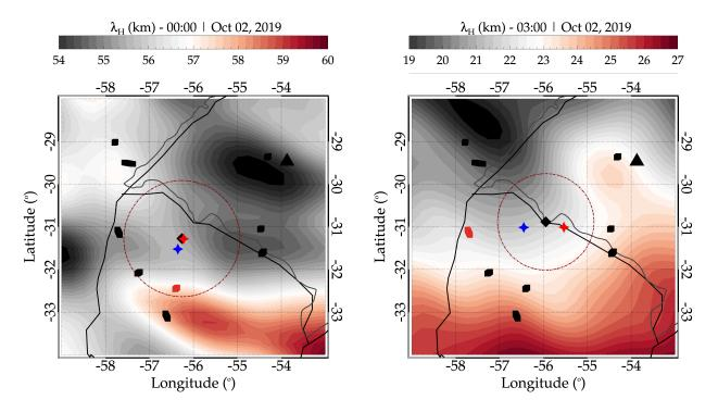
Figure 15. Horizontal wavelength spectra obtained using dispersion relation. In the left panel is the horizontal wavelength spectra above the tropopause between 00:00 and 01:00 UT whereas, between 03:00 and 04:00 UT is shown in the right panel.
