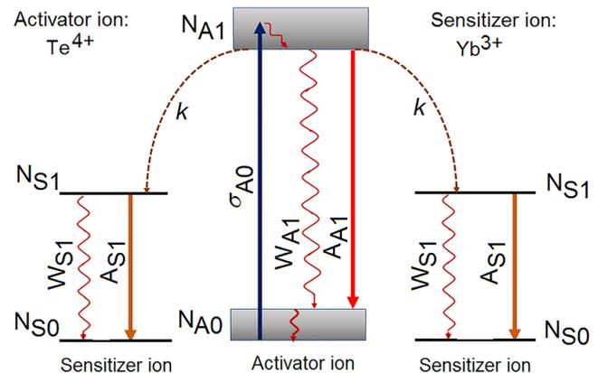
FIG. 16. Partial energy level diagram of an activator (Te<sup>4+</sup>) ion and two sensitizer (Yb<sup>3+</sup>) ions. The solid arrows and the wavy lines represent the radiative and non-radiative transitions, respectively. The dash arrows indicate the cooperative energy transfer (CET) mechanism for the near infrared quantum cutting emission under UV-blue excitation.
