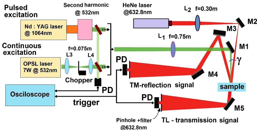
FIG. 14. Experimental setups for CW or pulsed lasers in the mode-mismatched configuration for the TL and TM methods.<sup>107,108</sup>
