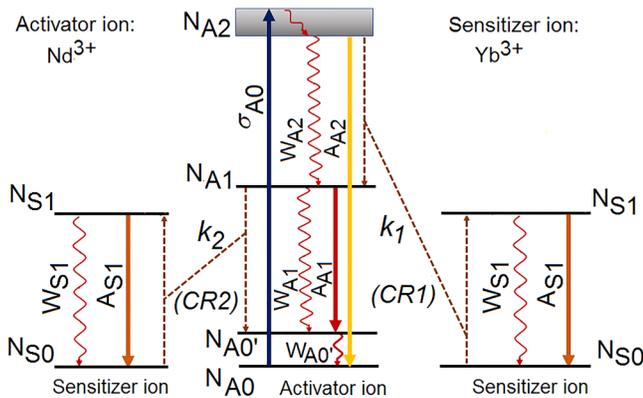
FIG. 18. Partial energy level diagram of the activator ( $\text{Nd}^{3+}$ ) and two sensitizer ( $\text{Yb}^{3+}$ ) ions. The solid arrows and the wavy lines represent the radiative and non-radiative transitions, respectively. The dashed arrows indicate the cross relaxation (CR) mechanism.
