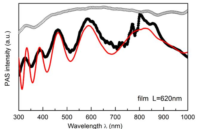
FIG. 12. Photoacoustic spectra (PAS) of the (o) c-Si substrate and (•) glass thin film deposited on the c-Si substrate. The solid line shows the PAS theoretical simulation using Eq. (9).
