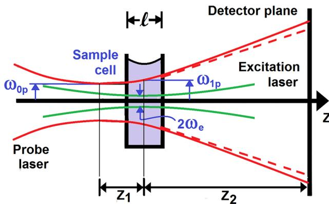
FIG. 13. A schematic diagram of the geometric positions of laser beams in a mode-mismatched dual-beam TL experimental arrangement.
