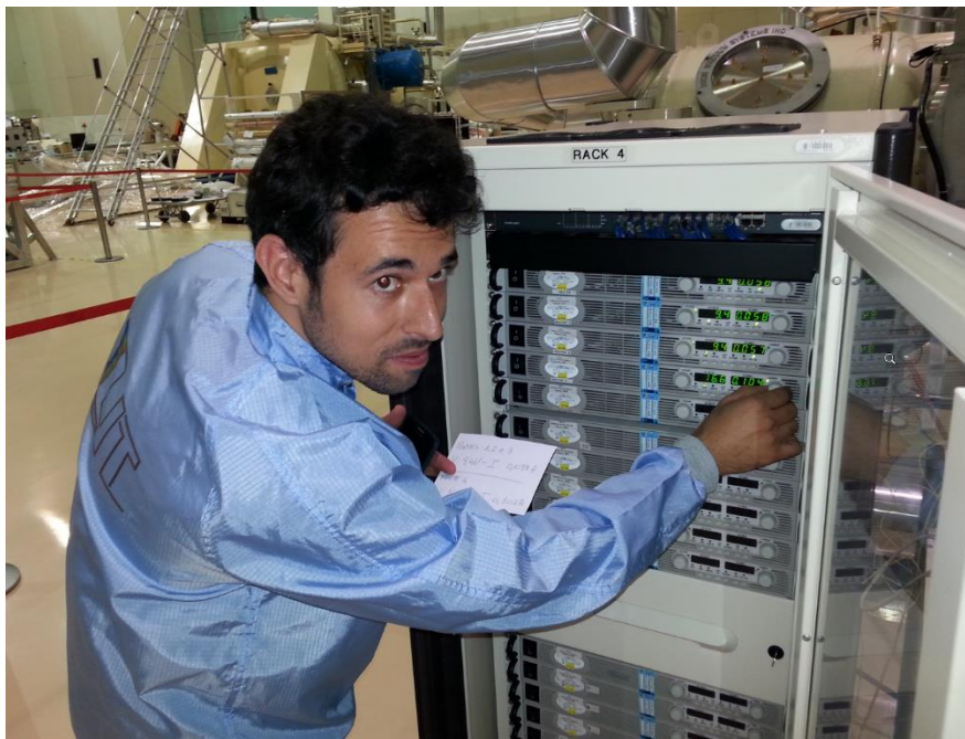
Figure C.4 – Test execution, OSRA heater power tuning.
