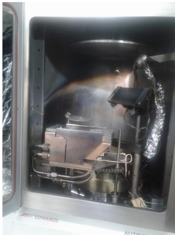
Figure B.1 – Electron Beam Vacuum Chamber.
