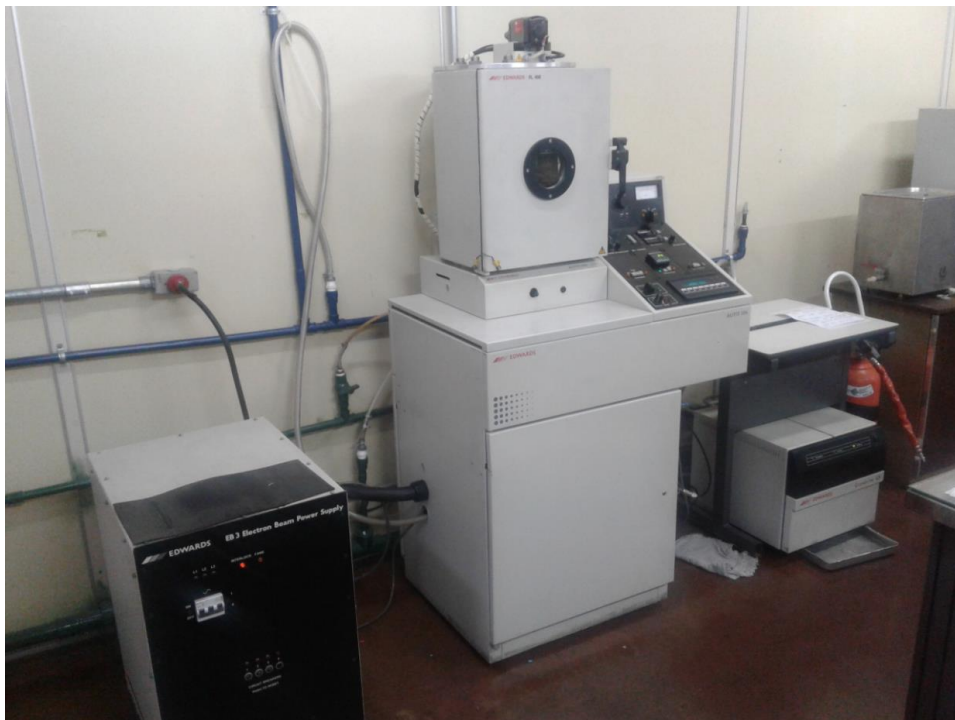
Figure B.4 – E-beam equipment used Edwards AUTO 306.
