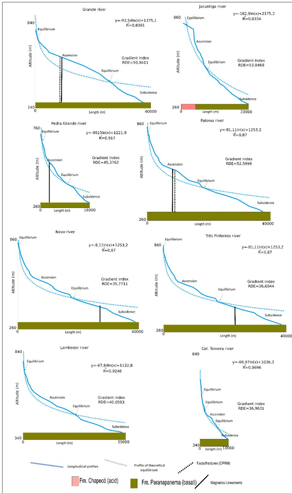
Figure 12. Longitudinal profiles of the rivers located on the left bank of the Uruguay River, that run entirely within the study area. (Elaborated by the authors)
