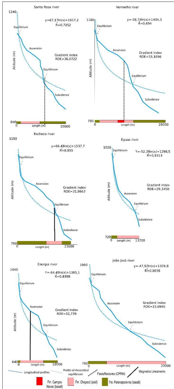
Figure 6. Longitudinal profiles of the right bank tributaries of the Chapecó River. (Elaborated by the authors)
