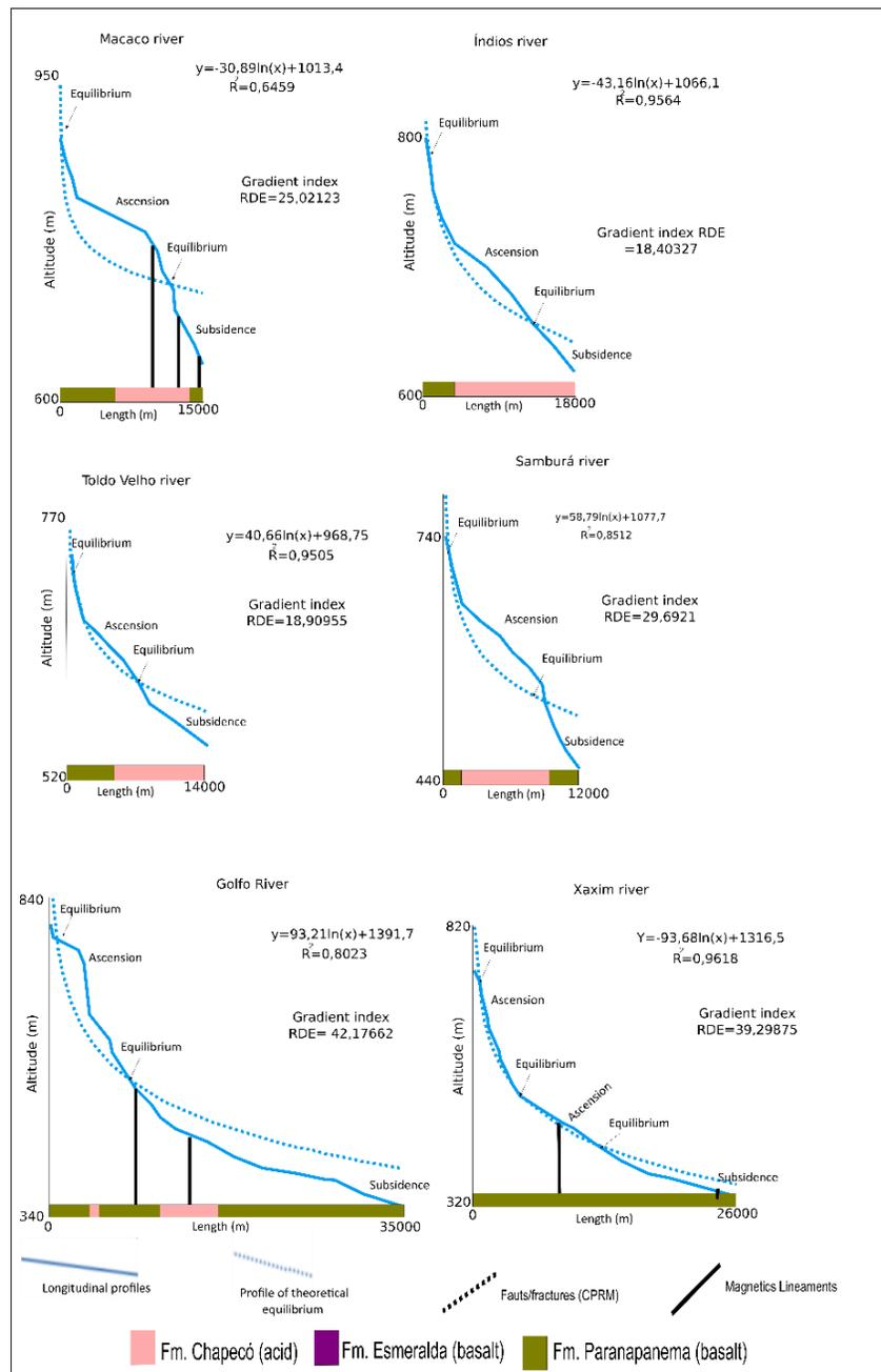
Figure 8. Longitudinal profiles of the left bank tributaries of the Chapecó River. (Elaborated by the authors)
