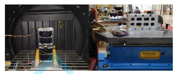
Figure 4: The NANOSATC-BR2 mounted with several internal and external thermocouples inside the Thermal Vacuum Chamber (left), and the CubeSat placed inside a Test-POD on a shaker at the Integration and Tests Laboratory – LIT / INPE - MCTI (right) (Asencio, 2021).
