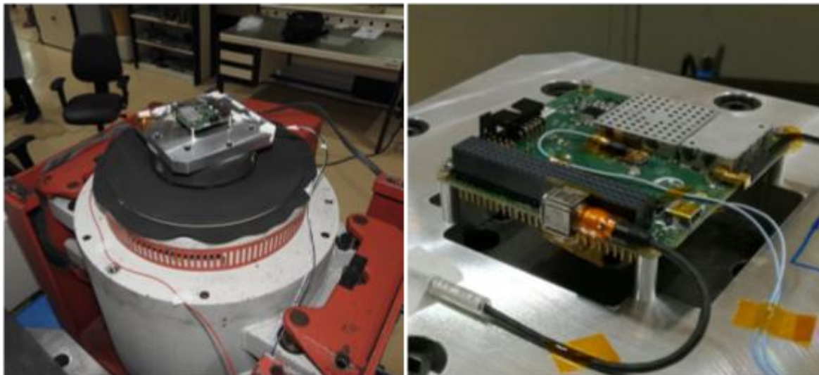
Figure 4: EDC Mechanical Vibration Test.
