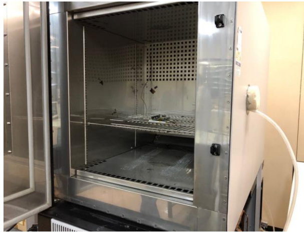
Figure 5: EDC in the Climatic Chamber for the thermal cycling test.
