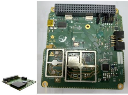
EDC - Environmental Data Collection Transponder
