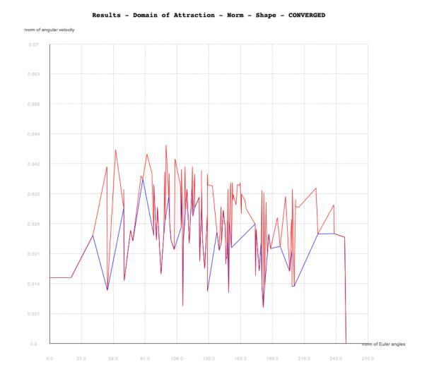
Figure 3: ROA with nonlinearities in the reactions wheels.
