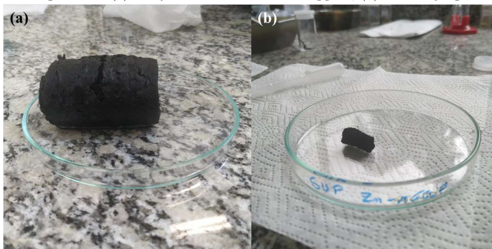
Figure 4.3 - (a) As-synthesized Zn-rGO_P support; (b) After drying.
