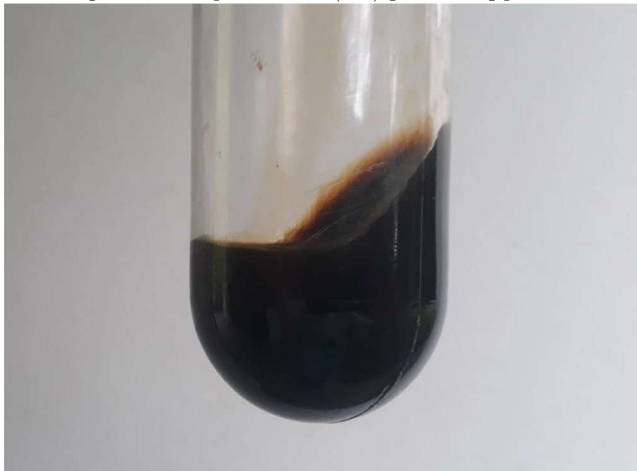
Figure 4.2 - Graphene Oxide (GO) gel resulting product.
