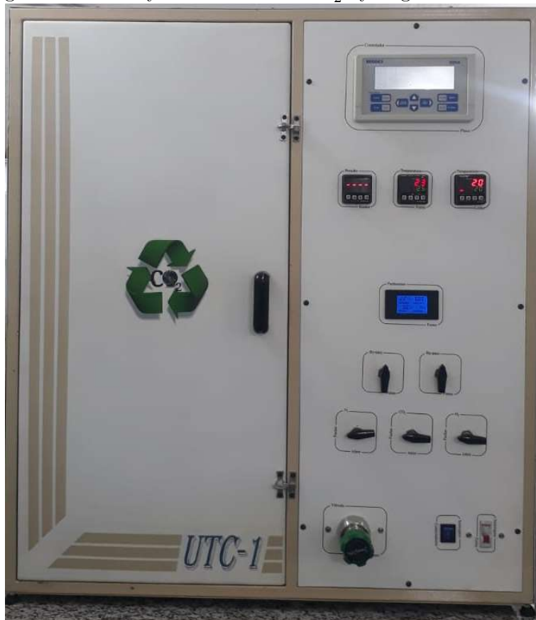
Figure 3.7 - Catalytic Unit for the CO 2 hydrogenation reaction.
