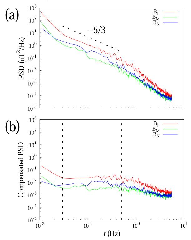
Figure 4. (a) PSD of the  $B_L$ ,  $B_M$ , and  $B_N$  components of the magnetic field (event 1). (b) Compensated PSD. The dashed vertical lines indicate the inertial subrange in which the compensated PSD is nearly horizontal.
