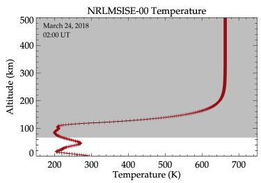
The dark red plus sign shows the profile at each 1 km. The gray shaded region ranges from 65 to 500 km which emphasizes the range of NRLMSISE-00 temperature profile to be used for the concatenation.
