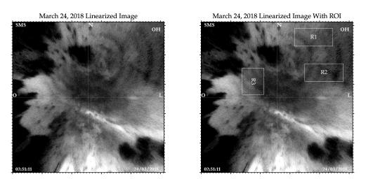
Illustration of all-sky images with visible concentric dark and bright bands (left panel). In the right panel, regions of interest ( $R_1$ ,  $R_2$ , and  $R_3$ ) selected to be used in the spectral analysis.
