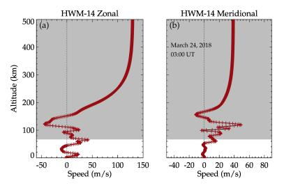
The dark red plus sign shows the profile at each 1 km. In panel (a), the zonal wind is shown whereas the meridional wind is shown in panel (b). The gray shaded region ranging from 65 to 500 km indicate the altitude range of the HWM-14 wind profile to be used in the concatenation. The vertical dotted lines demarcate the direction of the winds. Positive for north and east, and negative for south and west.
