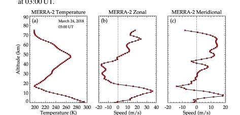
Figure 3.19 - Vertical horizontal wind profile obtained from MERRA-2 model for March 24, 2018, at 03:00 UT.
