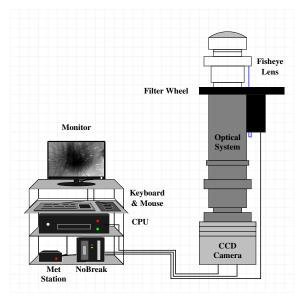
The imager is composed of an optical system, interference filters, CCD camera, computer system, power supply and the instrument's meteorological station (MetStation). Source: Adapted from Wrasse (2004).
