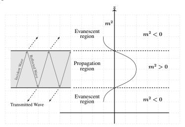
Figure 2.4 - Profile of the vertical wavenumber in the case of a duct.
