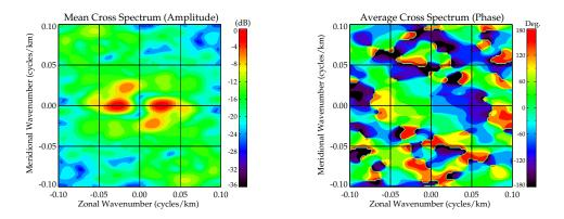
the amplitude of the cross-spectrum is the same result as the power spectrum shown in Figure 4.4. In addition to the amplitude, the cross-spectrum also provides the phase of the spectrum shown in right panel of Figure 4.5. In the case where  $\Delta \varphi < 0$  for  $k_{max}$  and  $l_{max}$ , the unambiguity in the gravity waves propagation direction is shown in Figure 4.6.
