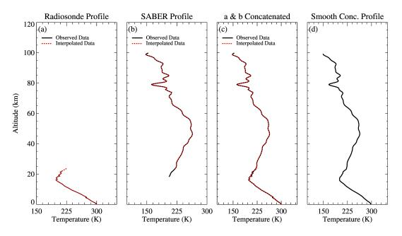
In panel (a) is the radiosonde profile, panel (b) is the SABER profile, and panel (c) is the concatenated profiles from (a & b). In panel (d) the final concatenated profile smooth at each three-point is shown. The black solid line and the red dashed lines in panels (a), (b), and (c) show the observed and interpolated profiles. respectively.
