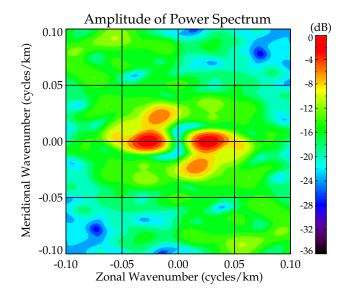
Positive wavenumbers represent the northward propagation direction for the meridional component and the eastward direction for the zonal component.
