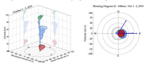
Figure 7.5 - 3D and 2D wind blocking diagram for the night of October 1 - 2, 2019.
