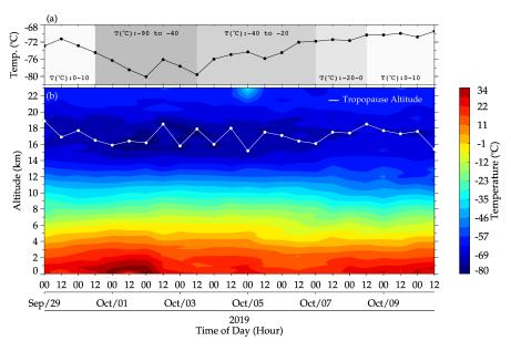
In panel (a), the variations of the tropopause temperature (black solid line with dots) along the days are presented. The grayscale regions with the label " $T(^{\circ}C)$ " represent the cloud top temperature range. The contour plot in panel (b) shows the temperature profile from 0-23 km at each 1 km along the days considered. The white solid line with dots shows the variations of the tropopause altitude with their respective temperatures shown in (a).
