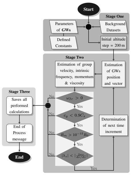
Figure 4.19 - Ray tracing model flowchart showing the stages of both backward and forward ray tracing.
