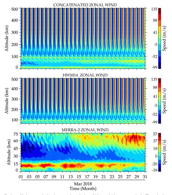
Each profile has a vertical and temporal resolution of 1 km and 1 hour, respectively. The color bars show the wind speed.
