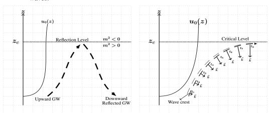
Figure 2.2 - A schematic diagram of reflection and critical/absorption levels of propagating gravity waves.
