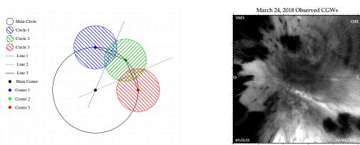
Left panel shows a diagram illustrating how the center and radius of a concentric (circle, ellipse and arc) pattern are determined using geometry technique. In the right panel, an observed CGWs on the night of March 24, 2018 at São Martinho da Serra is presented.
