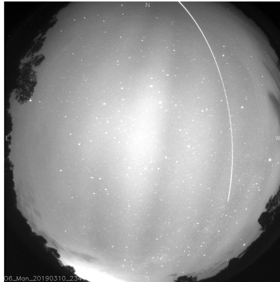
Figure 4.8 - On several occasions, the SWARM constellation path was observed on the field of view of all-sky imager at ZF-2 and one of the clearer ones was on March 10, 2019, at around 23:41:22 LT. The thin white line on the field of view is one of the satellites passing over the location of the all-sky imager.
