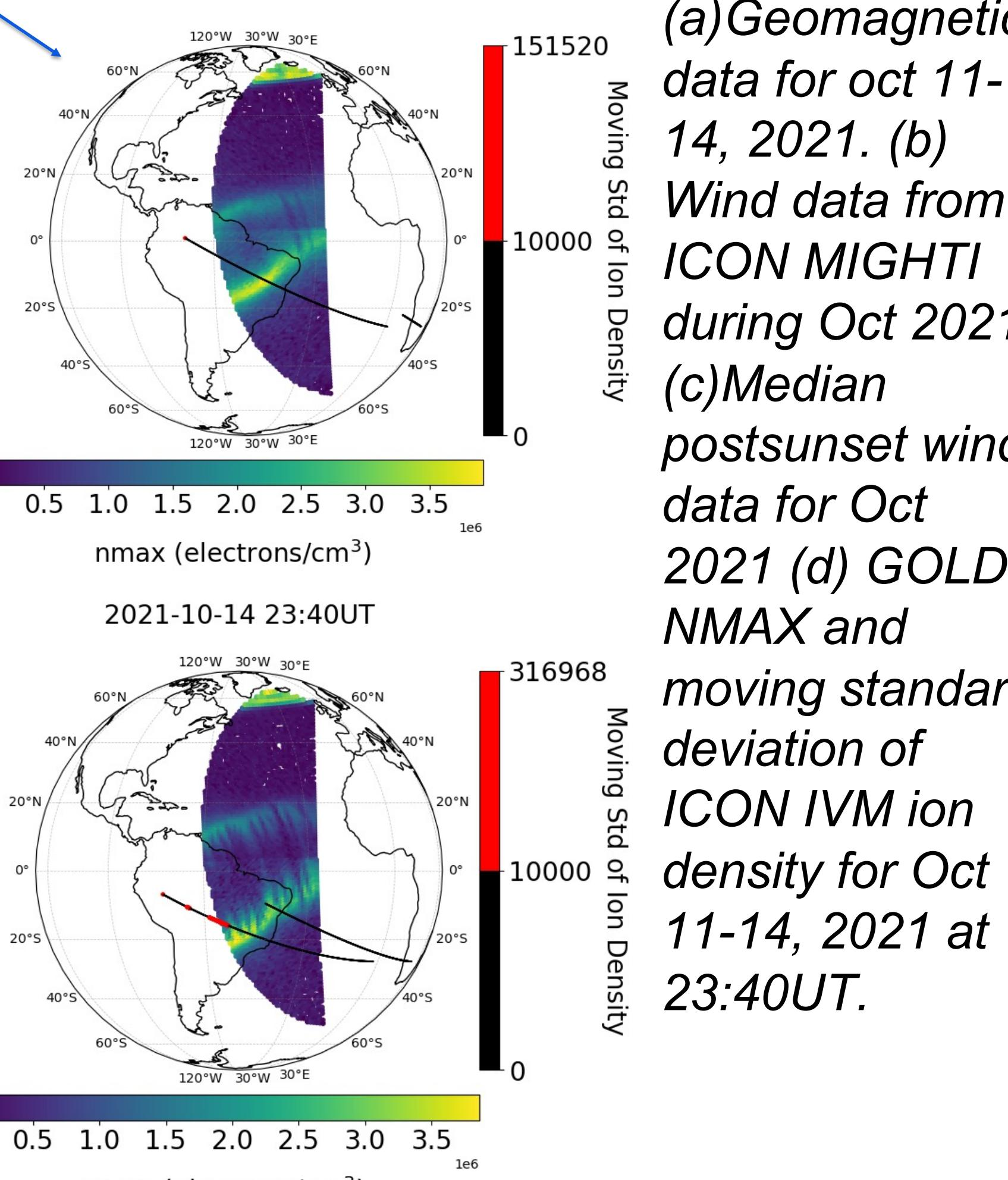
Plasma bubbles are usually observed at post-sunset over the Brazilian sector, but on post-sunset Oct 12 the bubbles were not detected (fig 1d). This was during the recovery phase of the geomagnetic storm occurred on Oct 12 (Fig 1a). Zonal wind (Fig 1b and c) turned eastward before the inhibition of the bubbles on Oct 12. The dotted lines indicate the period when the bubbles were inhibited.
