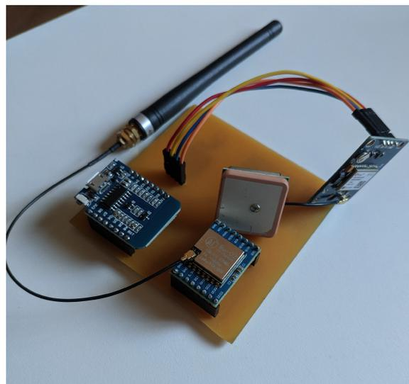
**Figure 3: PCB and Components Flight Segment Version 3.2.**
